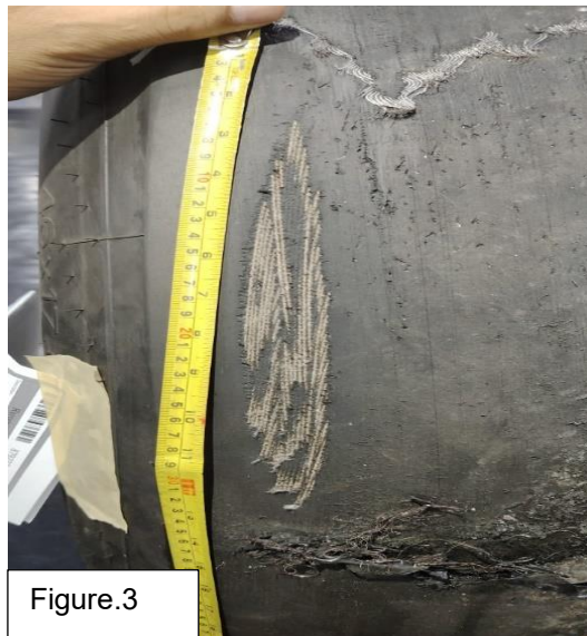
Figure 3 and 4: Showing damages sustained on the right main tires
