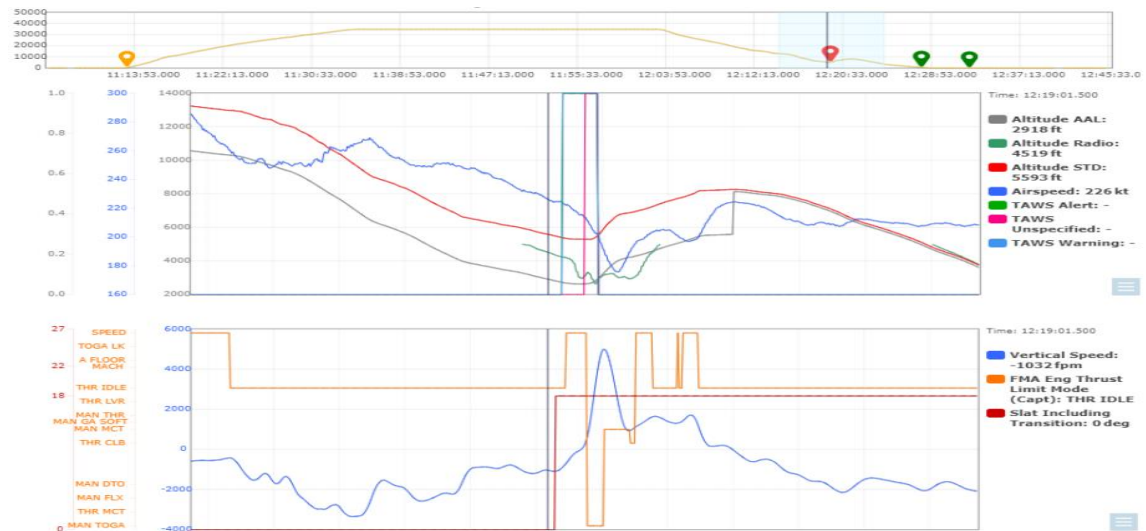
Figure 13 indicates TAWS warning, Vertical Speed and Thrust Mode (OMS104)
