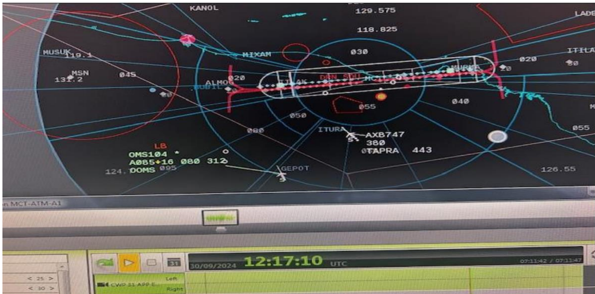
Figure 3: showing aircraft OMS104 observed on radar passing through 8500 Ft at ROD 1600 FPM descending to 8000 Ft (Source: DGAN)
