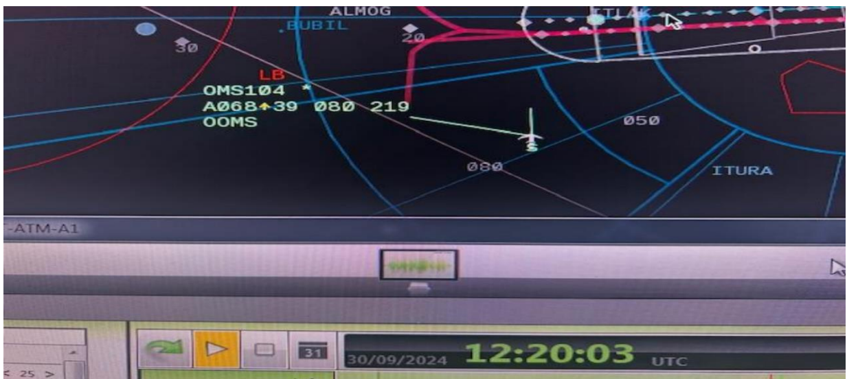
Figure 6: showing aircraft OMS104 observed on radar passing through 6800 Ft at ROC of 3900FPM climbing to 8000 Ft (Source: DGAN)
