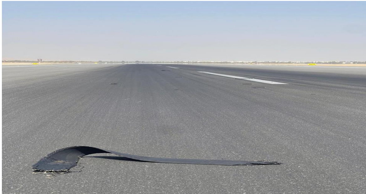
Figure 4: showing evidence of Main Wheel tire number 1 de-capped threat from the tire (Source: Oman Airports).
