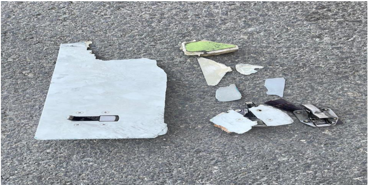
Figure 7: showing evidence of damaged access panel above left hand (LH) (Source: Oman Airports).
