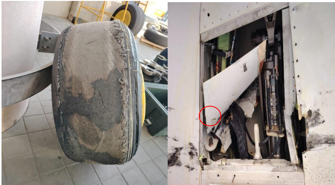
Figure 1 showing damages on the left-hand main tire, HYD pipes as indicated by red cycle and broken access panel.
