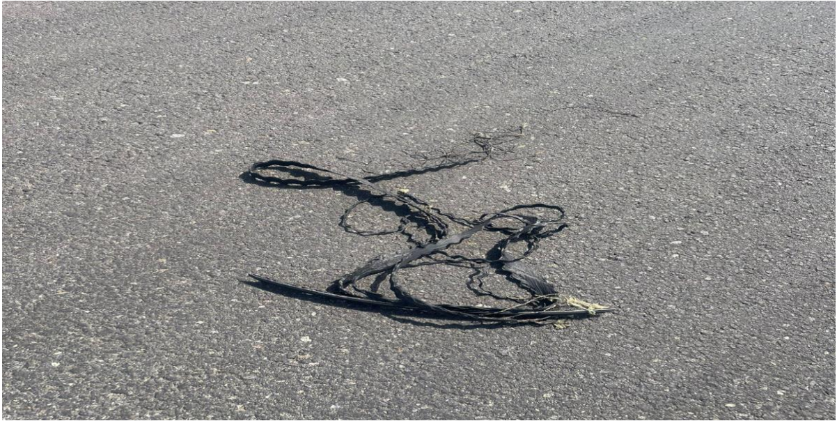
Figure 6: showing evidence of Main Wheel tire debris after tire de-capping (Source: Oman Airports).
